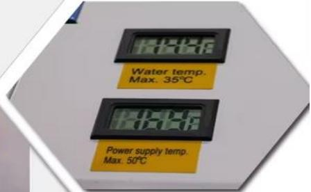
**9: Water temperature and laser power supply temperature display**
