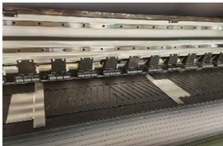
Honeycomb suction platform ensure the flatness of the paper more effectively when printing .
