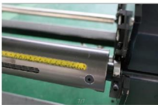
Inflatable take up and feed media shaft.
