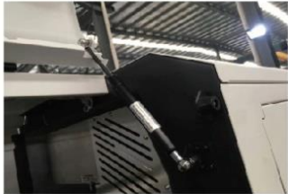
Machine cover increases cylinder control, More labor-saving and convenient .
